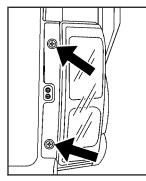
2. Remove the two screws from the taillamp assembly.
